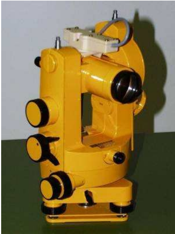
Fluxgate magnetometer mounted on a non-magnetic theodolite telescope.
