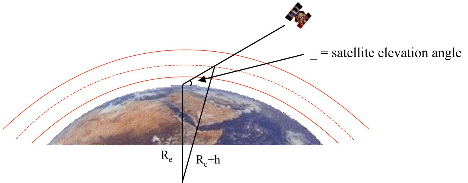
$$VTEC = \frac{1}{\sqrt{1 - \left( \cos \theta \frac{R_e}{R_e + h} \right)^2}} STEC$$
